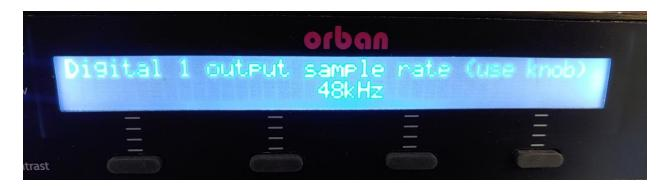
This option selects the sample rate of the AES output. Use the knob to select the correct sample rate and press NEXT.
