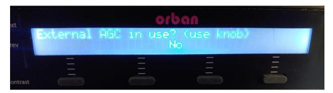
If you are using any pre-processing before the 5500i, you will want this to be set to YES. Orban recommends that no pre-processing should be used before the 5500i as the AGC in the 5500i is designed to work best with nearly all material and is crucial for optimum performance of your processor. However, if you feel the need to have an external AGC, you can turn the knob and select YES, the hit the NEXT key.
