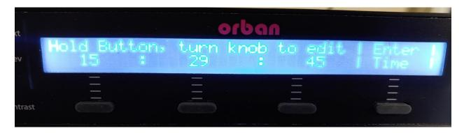
The first option is to set the time. The format is miliary time. Under each number is a button. Holding the button down while turning the knob will advance the HOURS, MINUTES or SECONDS. Once the correct time is set, press the ENTER TIME button.
