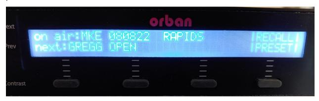
The processing screen top row will show the current preset on the air. Turning the knob changes the NEXT option to a different preset. In the example above, GREGG OPEN is the preset you want to put on the air. To do so, use the button under RECALL PRESET to change to GREGG OPEN.
