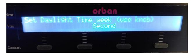
On this screen, use the knob to set the week daylight saving time will occur. When seleted, push the NEXT button.
