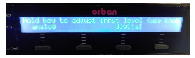
Hold down the button underneath the option and use front panel knob to set the ANALOG or DIGITAL input reference level. If you have audio hooked up to the 5500i, you should set this so that the AGC is showing approximately 9-12dB of gain reduction if the console or device feeding it is set to its normal operating level.
