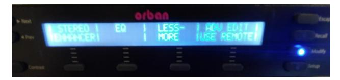
You will see four options. Stereo enhance sets the amount of additional enhancement you want to apply to the processing. A word of caution. If you are in an area prone to multipath distortion, you will want to tread lightly here as excessive enhancement can aggrivate or make the blend-to-mono effect in automobiles more noticeable. To access STEREO ENHANCER just push the button below the option. To exit, press the MODIFY button which will be illuminated.
