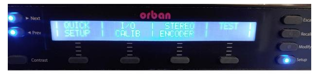
Pressing the SETUP button (the bottom button to the right of the screen) will enter this mode. There are four options here. These are all explained in the main Optimod 5500i manual, but for now we will deal with the first option, which is the Quick Setup.
