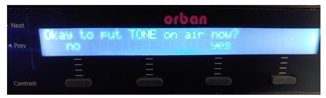
Gives you the option to put a tone on the air to set the proper modulation level. You can do this via tone, or you can use program material and watch the modulation monitor for overshoots. The 5500i has state-of-the-art overshoot protection, so once the modulation is set, all material will be held to that level or below.
