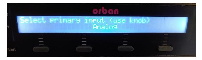
Use the front panel knob to select the corresponding main input signal. The options are ANALOG, DIGITAL and DIGITAL J17. Most will use ANALOG or DIGITAL. Once selected, press the NEXT button.
