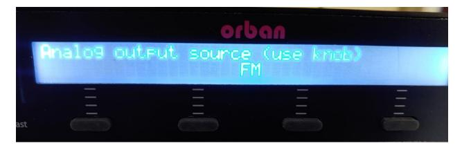
Use the front panel knob to route the audio you want to appear on the analog output XLR's. The options are FM or FM de-emphasized (where a de-emphasis filter to match the pre-emphasis selected earlier is applied). Once the output is selected, press NEXT.
