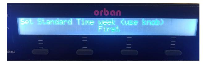
On this screen, use the knob to set the week daylight saving time will end. When seleted, push the NEXT button.
